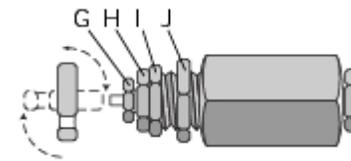
1. Hold "I" firmly and loosen nut "H".
